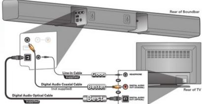
Most modern digital TV's do not have Red and White Coaxial Analog Audio Outputs, but do have Red and White Coaxial Analog Audio Inputs. If you plan to use Red and White Analog Coaxial Cables to Connect your TV to this Soundbar, please ensure that your TV does indeed have Red and White Coaxial Analog
