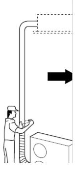
Do not wind the armoring tape too tightly since this will decrease the heat insulation effect. Also ensure that the condensation drain hose splits away from the bundle and drips clear of the unit and the tubing.
