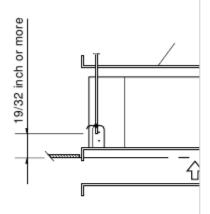
and the bottom of the ceiling of 19/32 in. or more as shown in Fig. 3-4.
