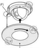
Place the cover on the ceiling and turn it clockwise to secure it.
