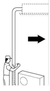
condensation drain hose splits away from the bundle and drips clear of the unit and the tubing.
