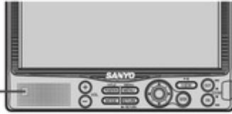
Do not cover the brightness sensor with a cloth. This will disable the detection of luminosity.
