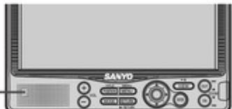
Do not cover the brightness sensor with a cloth. This will disable the detection of luminosity.
