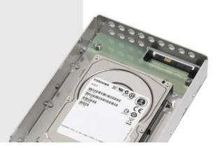
first of Toshiba's 10,000 RPM drives to employ a dual-stage head positioning actuator that provides additional performance gains, including a 32% increase in sustained transfer rate.
