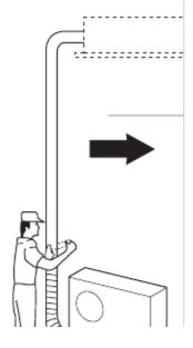
Do not wind the armoring tape too tightly since this will decrease the heat insulation effect. Also ensure that the condensation drain hose splits away from the bundle and drips clear of the unit and the tubing.
