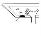
(2) Drill holes at the 4 points indicated on the fullscale diagram.
